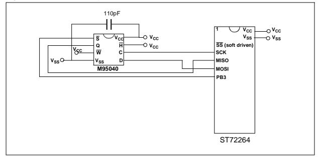
SS pin of ST72264 is software driven (high state for a master device).
